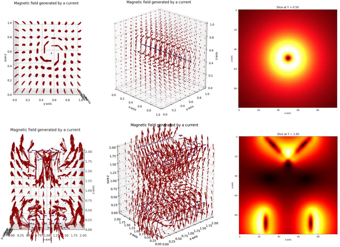
Figure 3: Output for the simulation of the magnetic field. **Top.** Magnetic field due to a linear current passing through space. **Bottom.** Magnetic field of the Stern Gerlach Device with vertical magnetisation. The plots on the left represent the magnitude of magnetic field at that point. The warmer the color the higher the magnitude
