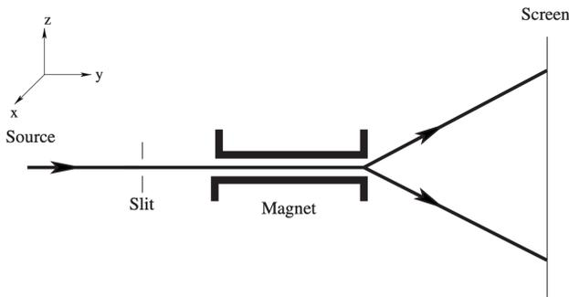
Figure 1: Stern Gerlach Device schematic. Incoming beam of particles focused from an oven source, passing through a magnetic field, will end up in separation according to the particle's spin. Adapted from [1]
