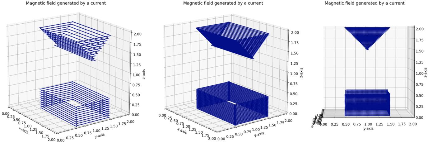
Figure 2: Generated mesh of Stern Gerlach Device magnet. Perpendicular uniform magnetisation is assumed. The blue arrows represent virtual surface currents.
